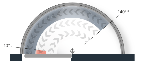
Closing force diagram ECO Newton TS-31, opposite hinge side
