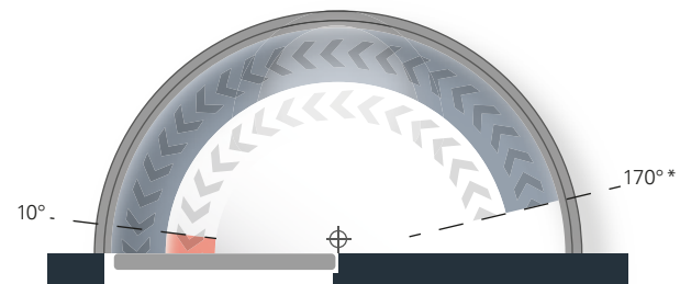
Closing force diagram ECO Newton TS-15, opposite hinge side
