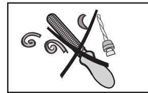
Bore chips seize latch and dead bolt
